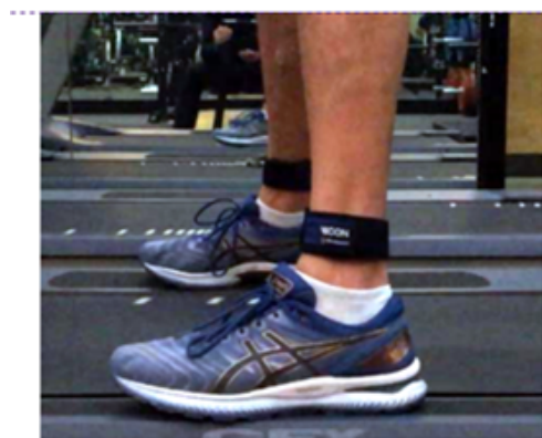
Figure 1. Example placement of the IMU device on the ankle.
