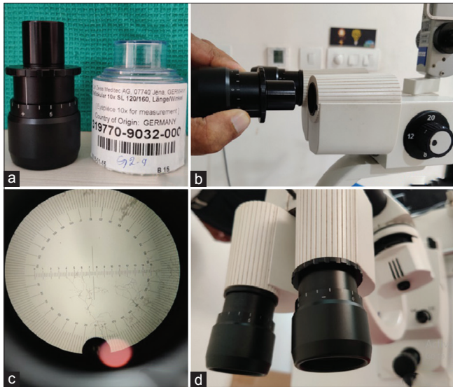
Figure 2: (a) Reticle incorporated eyepiece. (b) Inserting reticle after removing the right eyepiece. (c) View through reticle incorporated eyepiece (d) Reticle mounted onto slit lamp
