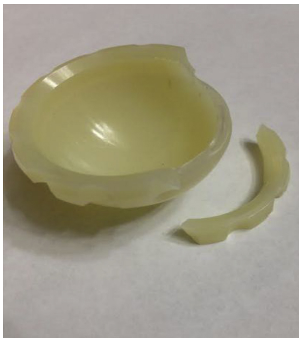
Figure 4. Photograph of fractured polyethylene component at the superior rim into 2 fragments with no visible thinning of the liner.
