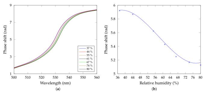
**Figure 10.** (a) Measured phase shift as a function of the wavelength for the increasing air humidity. (b) Measured phase shift as a function of the relative humidity with a polynomial fit ( $R^2 = 0.9965$ ). Wavelength is  $\lambda = 532$  nm.
