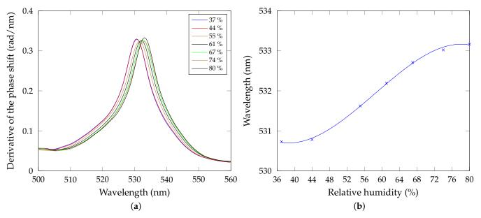
**Figure 11.** (a) Derivative of the phase shift as a function of the wavelength for the increasing air humidity. (b) Wavelength of the extreme of the derivative of the phase shift as a function of the relative humidity with a polynomial fit ( $R^2 = 0.99765$ ).
