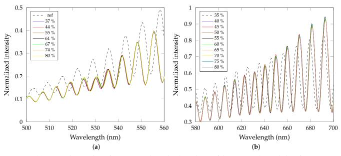
**Figure 9.** (a) Measured spectral interferograms involving the phase change of the BSW together with the reference one. (b) Measured spectral interferograms involving the phase change of the GW2 together with the reference one.
