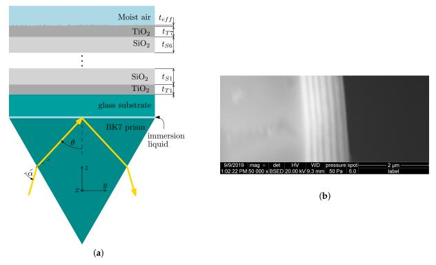
Figure 1. (a) A coupling prism with a photonic crystal under consideration. (b) SEM image of the photonic crystal.
