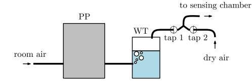
Figure 8. System to control the RH of air, including peristaltic pump PP and water tank WT.
