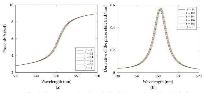
**Figure 6.** (a) Theoretical phase shift as a function of the wavelength with the increasing fraction of water *f* in the effective medium layer. (b) Derivative of the phase shift as a function of wavelength.
