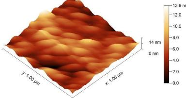
Figure 2. A topography image obtained by an AFM measurement.
