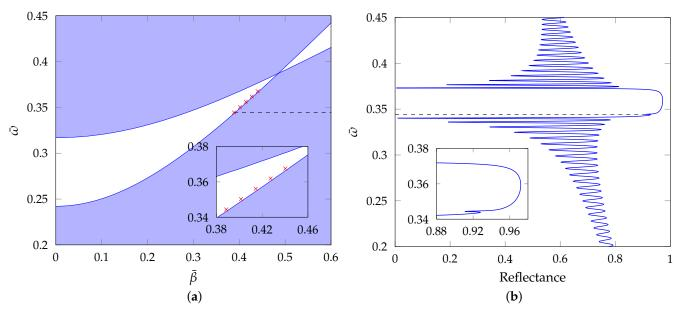
**Figure 4.** (a) A band diagram of an infinite multilayer structure. Red crosses are related to the Bloch states. Inset shows positions of the resonance states in detail. (b) Reflectance of the structure with 100 bilayers as a function of  $\bar{\omega}$ . Light is *p*-polarized, angle of incidence is  $\theta = 48^{\circ}$ . Inset shows a shallow resonance dip related to the Bloch surface wave.
