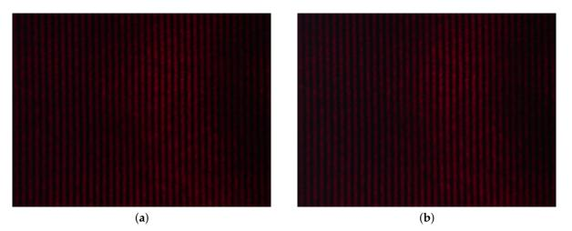
Figure 13. Recorded interference pattern obtained for the RH of 35% (a) and 80% (b).
