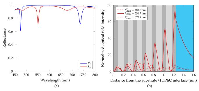
**Figure 5.** (a) Theoretical reflectance of the 1DPhC as a function of wavelength for both *p* and *s*-polarized light. The dip at a wavelength of approximately 551.5 nm is associated with the Bloch surface wave. (b) Normalized optical field distribution of *p*-polarized light in the structure. Angle of incidence  $\theta = 41.9^{\circ}$ .
