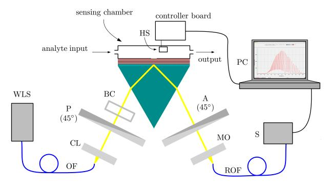
**Figure 7.** Experimental set-up consisting of white-light source WLS, optical fiber OF, collimating lens CL, polarizer P, birefringent crystal BC, a coupling prism with a multilayer structure and a sensing chamber, humidity sensor HS, analyzer A, microscope objective MO, read optical fiber ROF, spectrometer A and personal computer PC.
