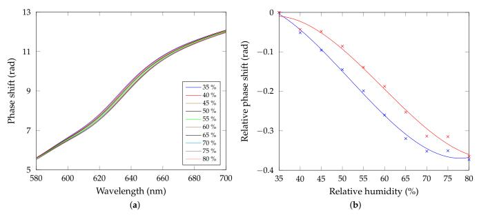
**Figure 12.** (a) Measured phase shift of the GW2 as a function of the wavelength for the increasing air humidity. (b) Measured relative phase shift as a function of the RH obtained by the spectral (blue) and spatial (red) phase detection methods with polynomial fits,  $R^2 = 0.9964$  (blue),  $R^2 = 0.9909$  (red).
