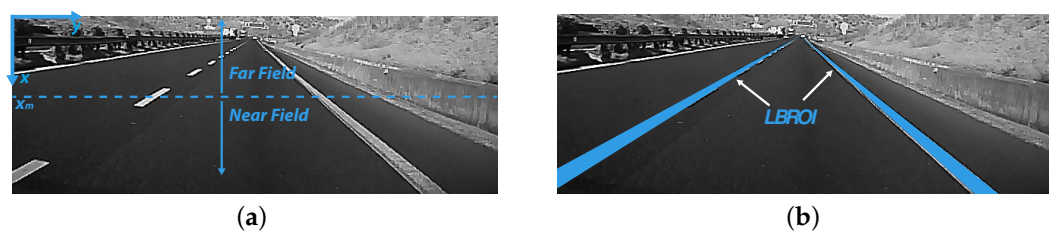
Figure 5. Linear–parabolic fitting: near and far field image separation (a) and LBROI (b).
