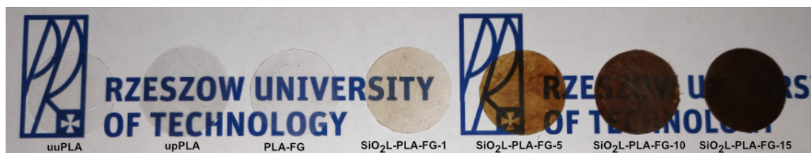
Figure 3. Visual appearance of SiO 2 -PLA-FG nanocomposites. PLA—polylactide, F—fusabond, G—glycerin.
