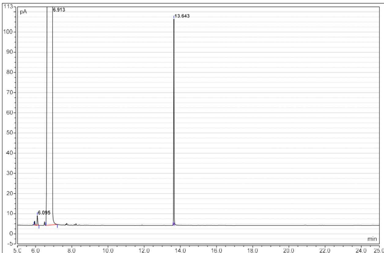
Figure 1. Gas chromatography of the crude mixture of the decarboxylation step (Table 2, entry 11). Propofol: t_R = 13.643 min, in the presence of the 2-butoxyethanol ( t_R = 6.095 and 6.913 min).
