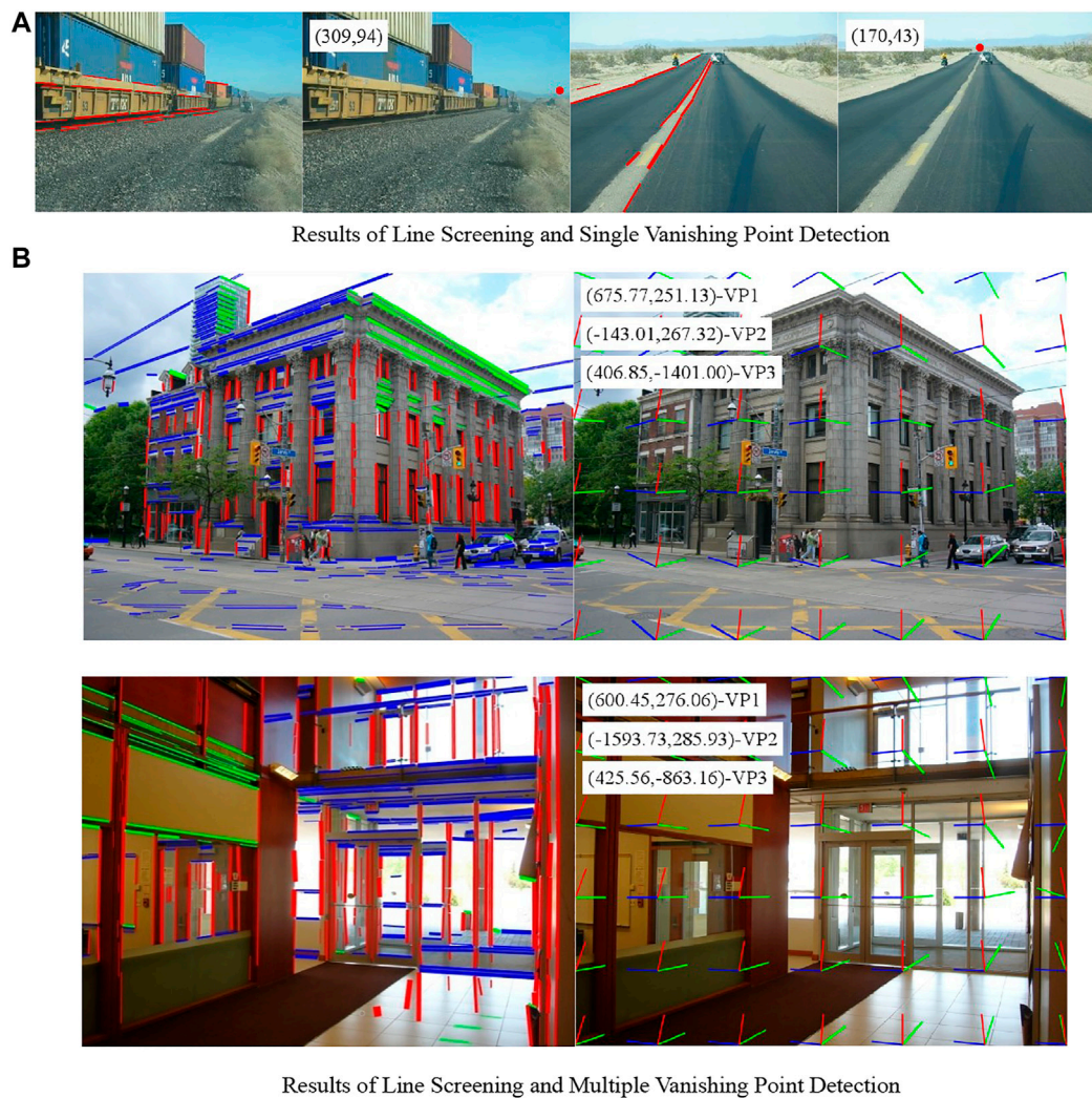
FIGURE 11 | Results of line screening and vanishing point detection. (A) Results of line screening and single vanishing point detection. (B) Results of line screening and multiple vanishing point detection.
