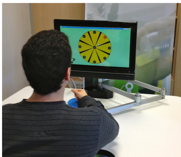
Figure 1 RoboTherapist 2D robotic device used in this study to monitor the reaching task.
