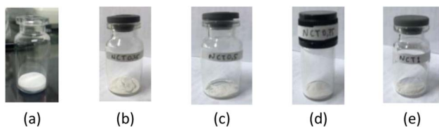
Fig. 2 Synthesized porous TiO 2 and N-doped porous TiO 2 nanoparticle samples: (a) CTO, (b) NCT0.25, (c) NCT0.5, (d) NCT0.75, and (e) NCT1.
