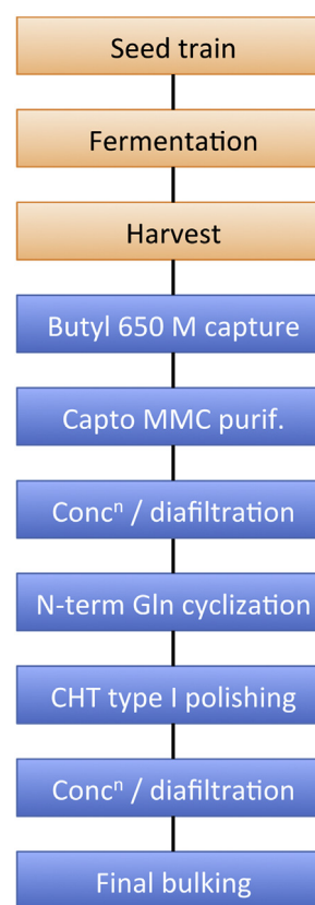
Fig. 5. Outline of scaled-up cGMP-compliant process to produce clinical grade recombinant 5P12-RANTES. Flow diagram indicating key steps in upstream (orange) and downstream (blue) processes. (For interpretation of the references to colour in this figure legend, the reader is referred to the web version of this article.)
