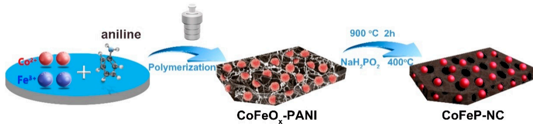
Scheme 1. Synthetic schematic diagram of the \text{CoFeP-NC} samples.
