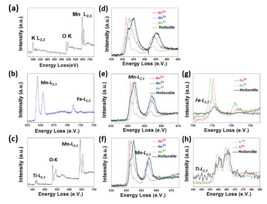
**Figure 13.** (**a**–**c**) EELS spectra characteristics of the undoped, and Fe-doped, and Ti-doped hollandites; (**d**) Mn  $L_{2,3}$  of undoped sample; (**e**) Mn  $L_{2,3}$  of Fe-doped sample; (**f**) Mn  $L_{2,3}$  of Ti-doped sample; (**g**) FeL<sub>2,3</sub> of Fe-doped hollandite; (**h**) TiL<sub>2,3</sub> of Ti-doped hollandite.
