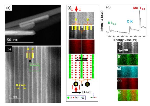
**Figure 9.** (a) Low-magnification STEM-HAADF image of several  $K_{0.12}$ MnO<sub>2</sub> nanowires; (b) HAADF image detail of a single nanowire; (c) from top to bottom: EELS spectra; online HAADF image, Mn chemical map; schematic model along the [110] direction; (d)sum spectra corresponding to the area framed in green in part b; (e) online HAADF image; (f) K-L<sub>2,3</sub> chemical map; (g) O-K chemical map; (h) Mn-L<sub>2,3</sub>; (i) K and Mn maps overlapped.
