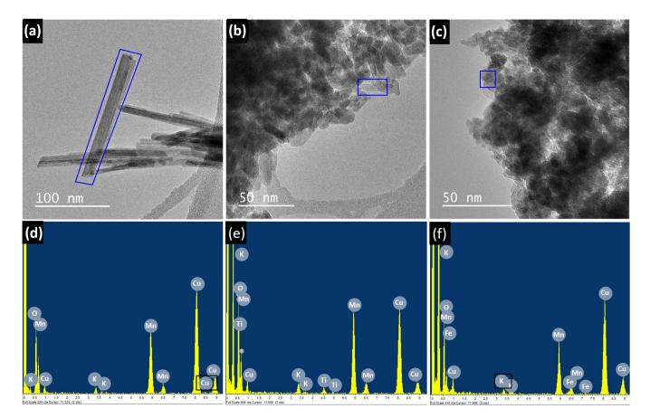
**Figure 5.** Low-magnification TEM images corresponding to the undoped sample (**a**); (**b**) the sample doped with 5% Ti; (**c**) the sample doped with 15% Fe; (**d**–**f**) corresponding EDS spectra.
