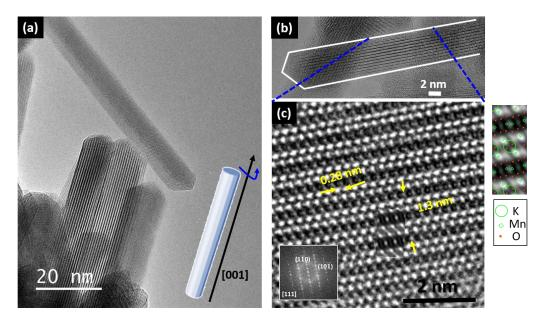
**Figure 7.** (a) High-resolution transmission electron microscopy (HRTEM) corresponding to several nanowires of undoped hollandite along the [11n] direction around the [001] direction as schematically represented in the model at the bottom-right; (b) image of one nanowire along the [111] direction; (c) atomically resolved detail and calculated image.
