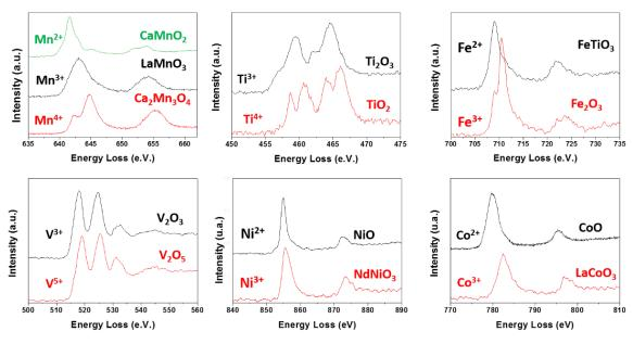
Figure 12. ML<sub>2,3</sub> edges for several oxides containing M = Mn, Ti, Fe, V, Ni, and Co in different oxidation states.
