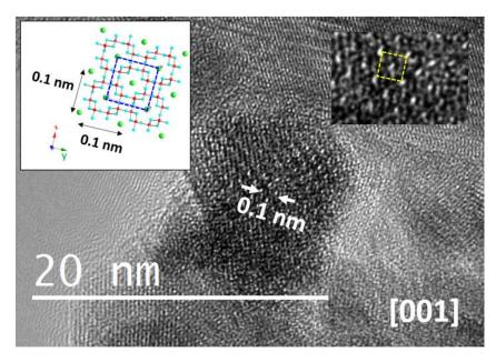
**Figure 8.** HRTEM image along the [001] direction corresponding to a 15% Fe-doped sample. An enhanced detail is shown in the right-upper part, and the schematic model along this projection is included in the left-upper part.
