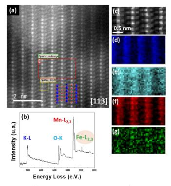
**Figure 10.** (a) STEM-HAADF image corresponding to  $K_{0.09}Mn_{0.88}Fe_{0.12}O_2$ ; (b) sum spectra of the area framed in green in a; (c) simultaneously acquired HAADF image; (d) K-L<sub>2,3</sub> chemical map; (e) O-K chemical map; (f) Mn-L<sub>2,3</sub> chemical map and (g) Fe-L<sub>2,3</sub> chemical map.
