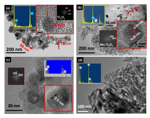
**Figure 4.** Characteristic low- and medium-magnification TEM images together with the typical EDS spectra of  $TiO_2$  reduced NPs (**a**); (**b**) Mn-doped  $TiO_2$ -reduced NPs; (**c**) ZnO-functionalized NPs; (**d**)  $\beta$ -FeOOH nanowires.
