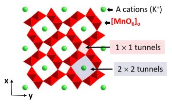
Figure 6. Schematic representation of the hollandite structure.
