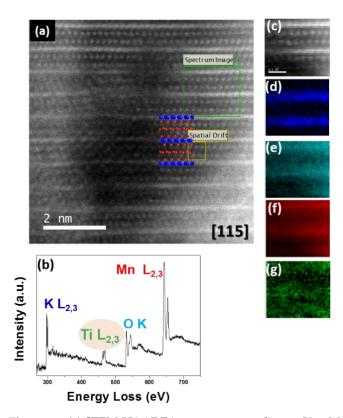
**Figure 11.** (a) STEM-HAADF image corresponding to  $K_{0.11}Mn_{0.92}Ti_{0.08}O_2$ ; (b) sum spectra of the area framed in green in (a); (c) simultaneously acquired HAADF image; (d) K-L<sub>2,3</sub> chemical map; (e) O-K chemical map; (f) Mn-L<sub>2,3</sub> chemical map and (g) Ti-L<sub>2,3</sub> chemical map.
