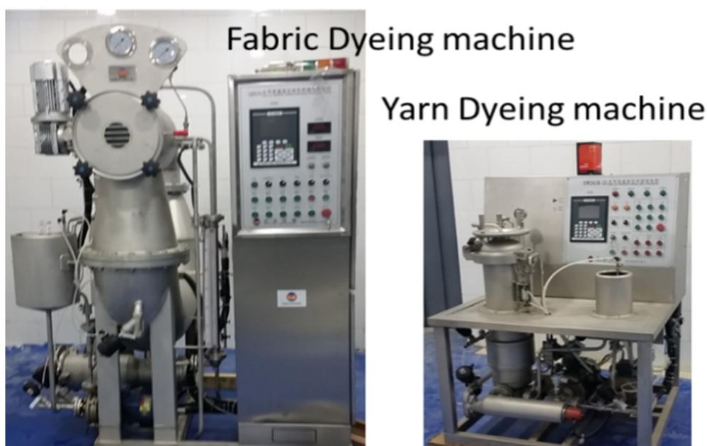
Fig. 1. Yarns and fabrics lab scale dyeing and finishing units.
