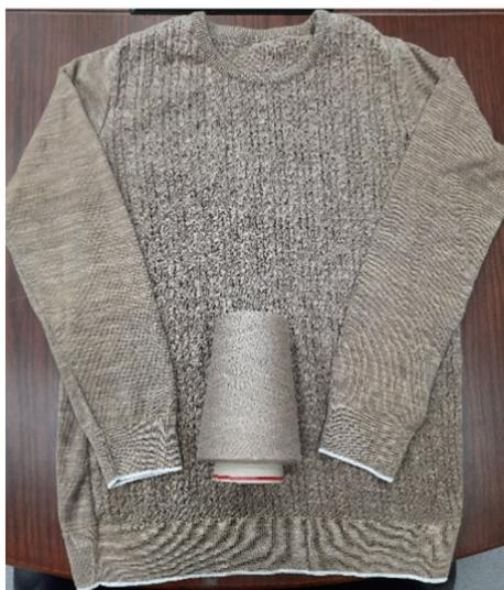
**Fig. 11.** Antimicrobial and antiviral winter sweater made of cotton yarns treated with AgNPs.
