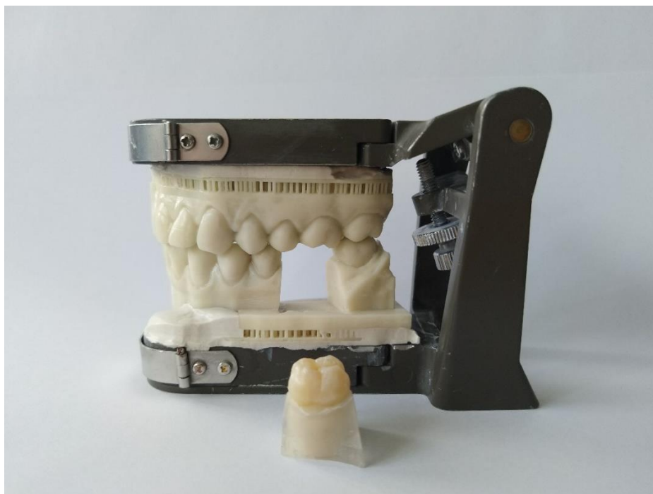
Figure 1. The test model with several interchangeable PMMA sockets and one of three different preparation geometries of the natural teeth ( n = 10 ).
