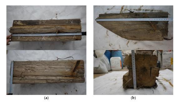
**Figure 5.** Samples and their dimensions: (a) sample 1 cross section  $18 \text{ cm} \times 20 \text{ cm}$  and length 60 cm, (b) sample 3 cross-section  $18 \text{ cm} \times 20 \text{ cm}$  and length 60 cm with cut.
