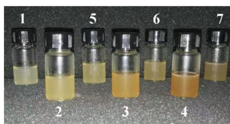
Figure 1. SF ink and SP composite ink prepared by G-SF, G-WS, and G-ILS. The number of SF ink and SP composite ink in the figure are (1) G-SF, (2) G-SF/WS (10%), (3) G-SF/WS (20%), (4) G-SF/WS (30%), (5) G-SF/ILS (10%), (6) G-SF/ILS (20%), and (7) G-SF/ILS (30%).
