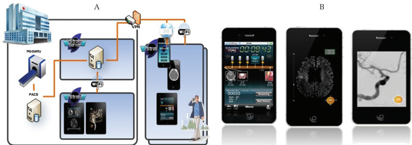
Fig. 1 (A) Components of the system (SYNAPSE Erm) for connecting off- and on-site medical care providers. (B) Display of the diagnostic and treatment data on mobile devices.
