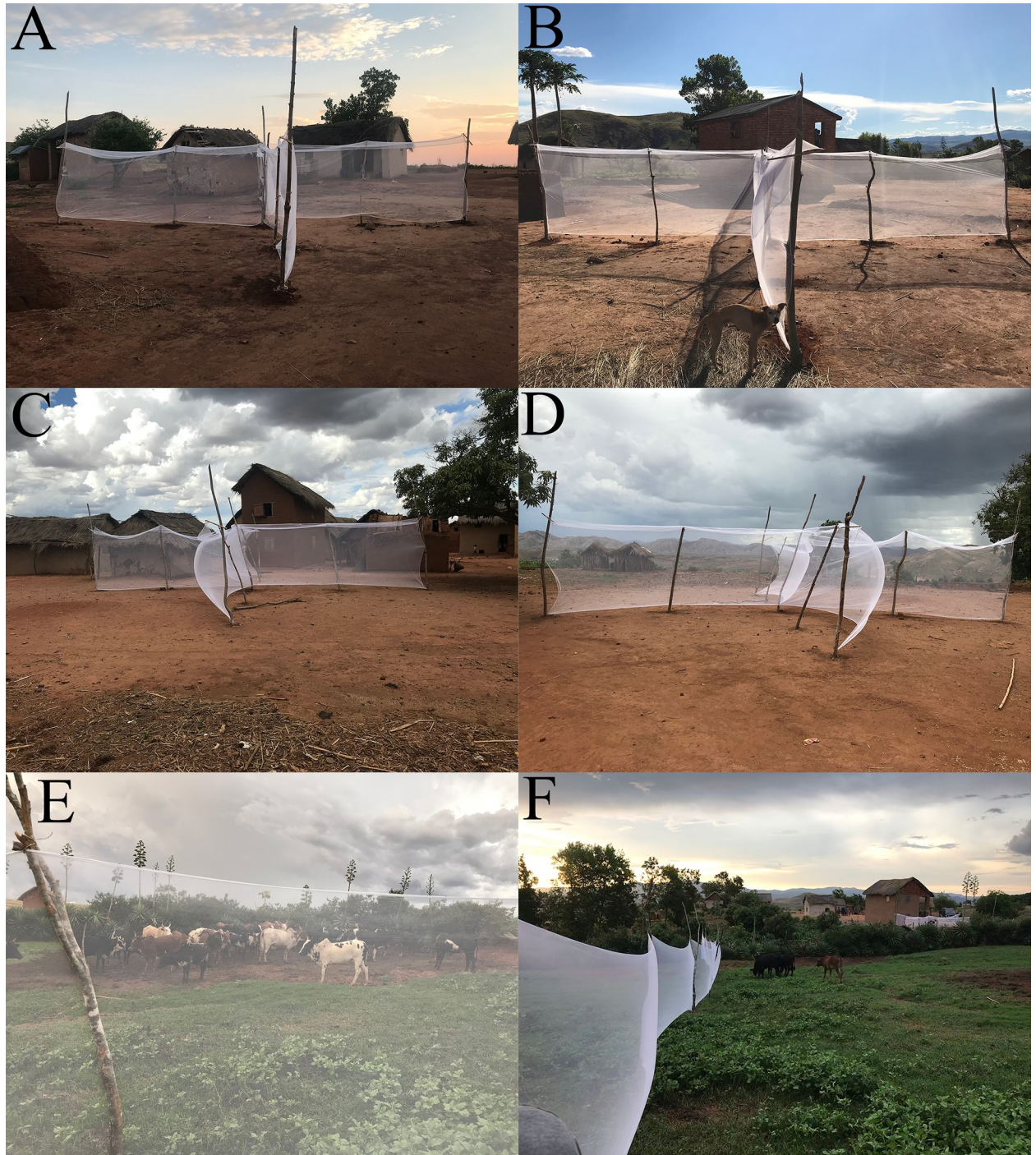
Fig 2. Quadrant Enabled Screen Trap (QUEST) with built-in eaves. A,B: Ambolodina T1. C,D: Amparihy T1. Standard Barrier Screen. E,F: Ambolodina T4.
