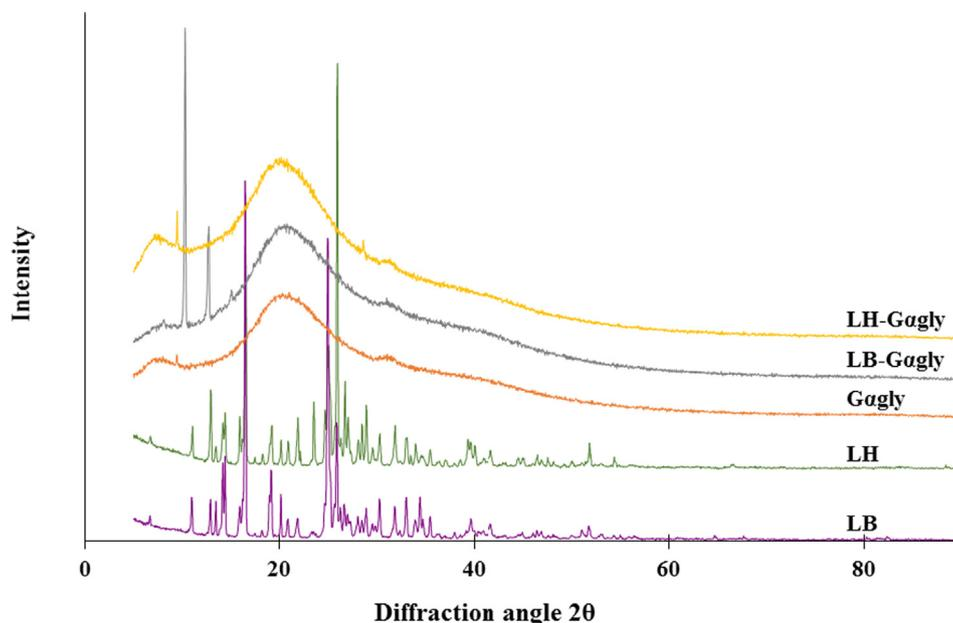
Fig. 4. XRD diffractograms of blank film and medicated films.
