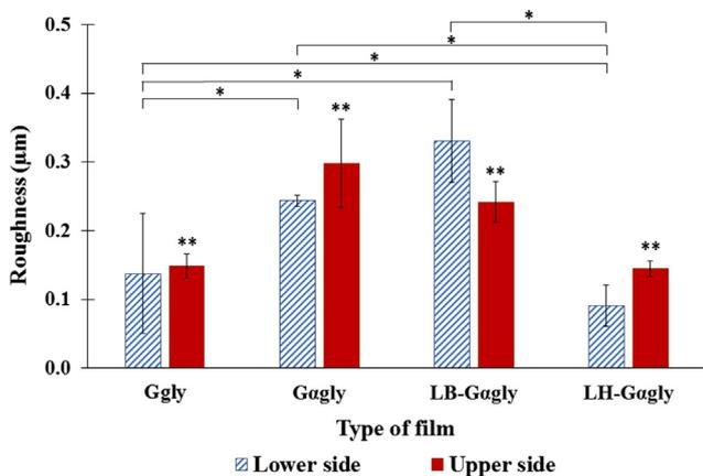
Fig. 2. The roughness values of the films calculated from AFM. \* meant the significant difference ( $p < 0.05$ ). \*\* meant each type of upper side film was significant difference ( $p < 0.05$ ).
