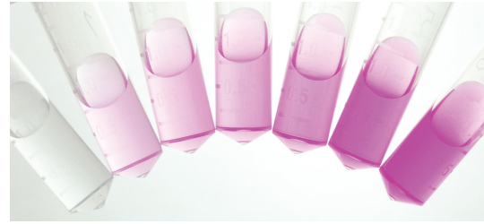
FIGURE 1: Increments to 0.1 \mu\text{L} (more left) to 0.7 \mu\text{L} (more right) added in 1.3 mL of the distilled water were used to compose the absorbance curve. The start point for this curve was the absorbance value of the water without addition of the color marker.
