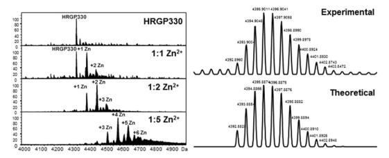
Figure 2. Deconvoluted ESI-MS spectra of HRGP330 incubated at varying  $Zn^{2+}$ :peptide ratios. Peptide samples (15  $\mu$ M) in 10 mM ammonium acetate (pH 7.40) were titrated with zinc acetate and were analysed on a maXis QToF mass spectrometer (Bruker Daltonics). The isotopic distribution for the 1:1 Zn-HRGP330 complex is shown on the right hand side together with a comparison to the theoretical model.
