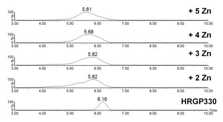
**Figure 4.** Effect of  $Zn^{2+}$  binding on the ATD of the 5+ charge state of HRGP330. ATD peaks of  $Zn^{2+}$  bound species, given in ms. The sample consisted of  $10\,\mu M$  HRGP330 in  $10\,m M$  ammonium acetate (pH 7.4) and  $50\,\mu M$  Zn. The  $Zn_1$ -HRGP330 peak identified in the sample was too low in intensity to give reliable data. The trace for the apo-peptide was acquired on a zinc-free sample. ATD data for all charge states for apo-HRGP330 are shown in Fig. S6.
