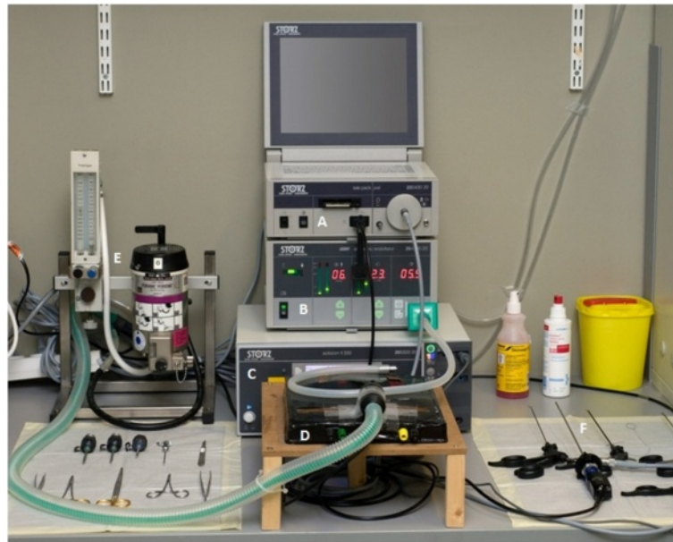
Figure 1 Animal operation workplace. (A) Tele Pack. (B) Electronic Endoflator®. (C) Autocon® II 200 (Karl Storz GmbH & Co KG, Tuttlingen, Germany). (D) Warming plate. (E) Equipment for anaesthesia. (F) 2- to 5-mm laparoscopic instruments (Karl Storz GmbH & Co KG).
