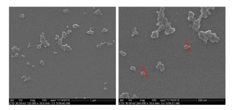
Figure 1. SEM microphotographs of SF/PEG nanoparticles.
