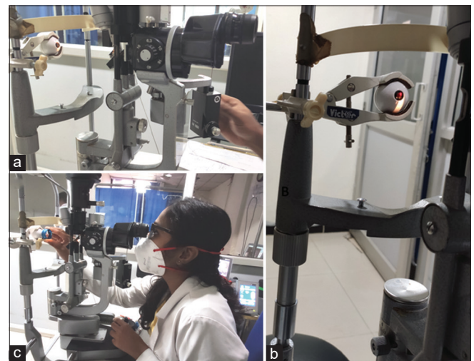
Figure 6: The 3D printed model eye is fixed in place using a metallic handle upon slit-lamp laser delivery system (a and b) A trainee practicing laser photocoagulation (c)
