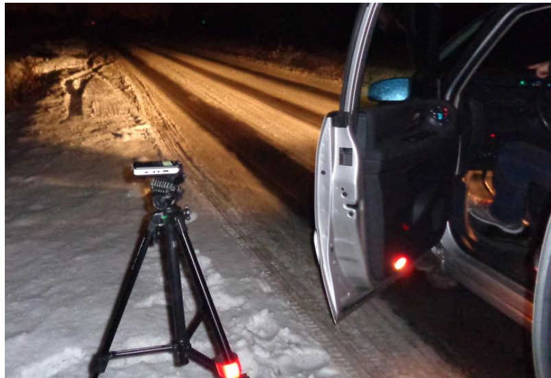
Figure 3. The road and the position of the audio recorder with built-in stereo microphones during on-road recordings in Lubartów in the winter.
