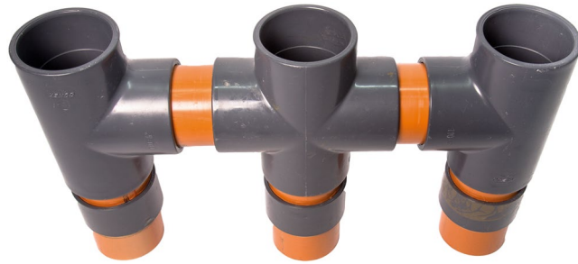
Figure 4. Plant growth system. 3.4L plant pots (110 mm diameter) are connected through a 1.2L (110 mm diameter) root-free chamber. Donor plant pot is at the center and connected to one receiver plant pot at each side. Photograph taken by Charlotte Knudsen.
