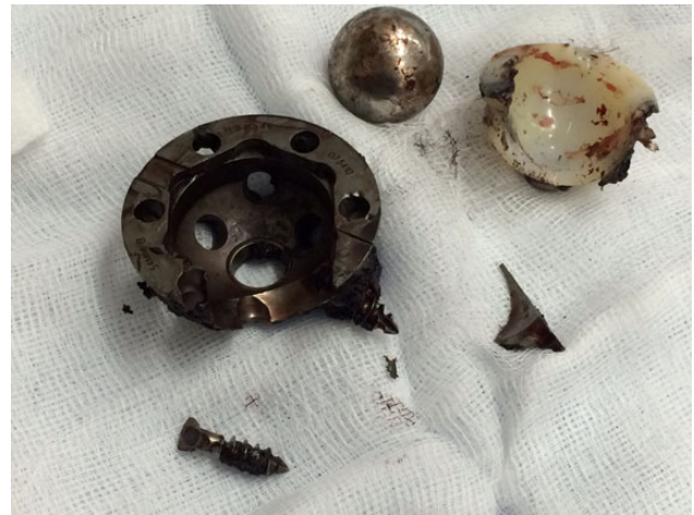
Figure 3: The acetabular component and liner showing extreme wear.
