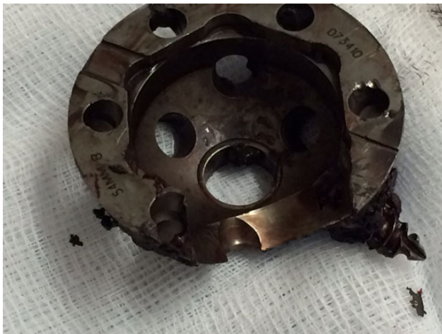
Figure 2: The acetabular component showing extreme wear-through and metallic fragments.
