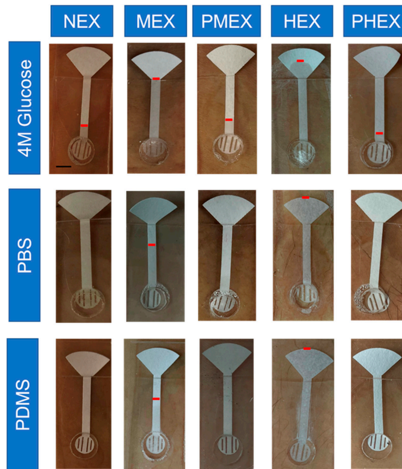
Figure 3. Optical images of the patch on skin showing the levels of sweat collection on the paper channel of patches with different pumping materials under different physiological conditions. The red mark on the paper channel indicates the position of sweat after each trial. Scale bar = 5 mm.
