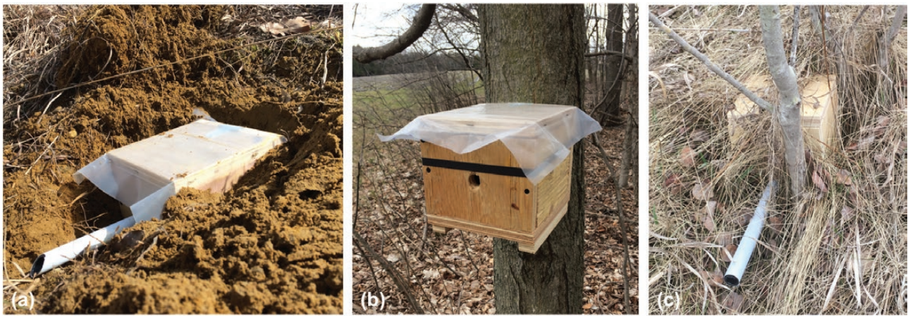
Fig. 2. Photographs of each domicile installation method: (a) underground domicile before complete burial, (b) aboveground strapped to tree, and (c) false-underground hidden in vegetation.
