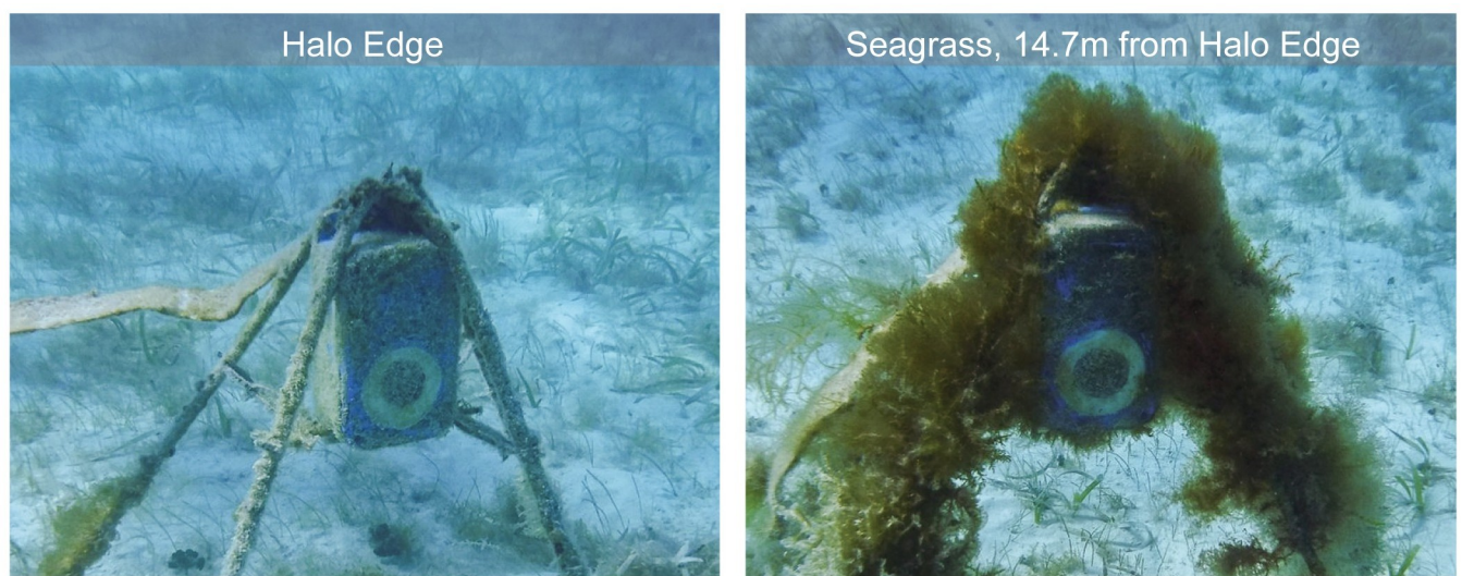
Fig 4. Comparison of biofouling and algal overgrowth after a month based on location. Structures were located at the edge of the halo, adjacent to seagrass (left), and in the middle of the surrounding seagrass (right). Similar results seen across all camera sites suggest that reef-based herbivores help to control algal growth both within and at the edges of the halo but do not graze heavily, if at all, on algae and related marine organisms in the surrounding algal or seagrass beds. Reprinted from [39] under a CC BY license with permission.
