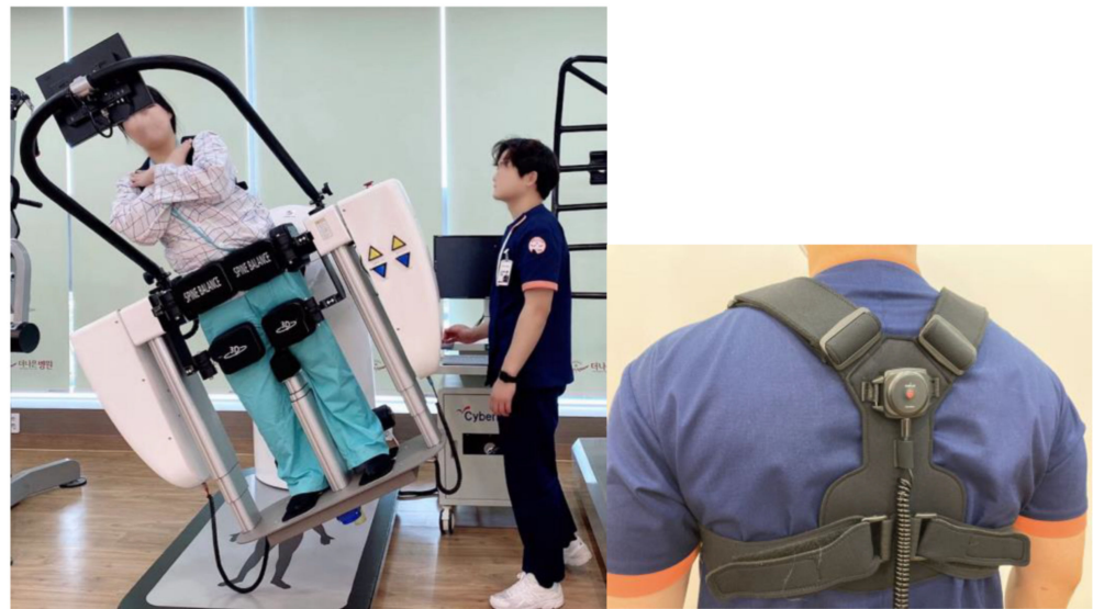
Figure 1. Spine Balance 3D. (left) Body tilt device, (right) inertia measurement unit (IMU) sensor.
