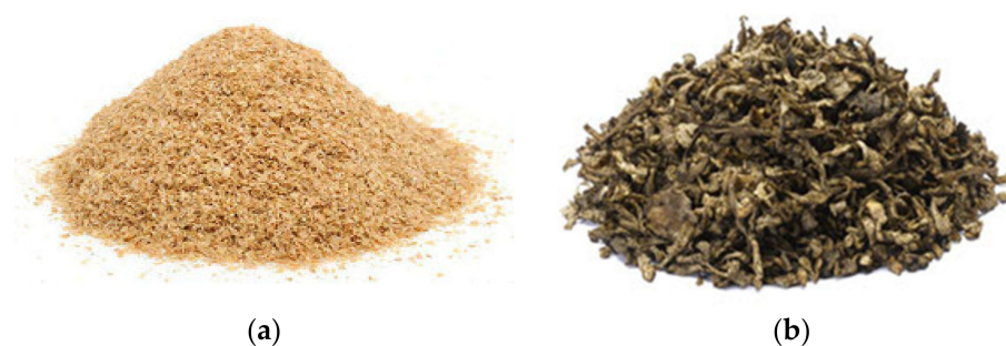
Figure 2. Agricultural waste used in the combustion process in the biomass low-power boiler: (a) wheat bran and (b) beet pulp.
