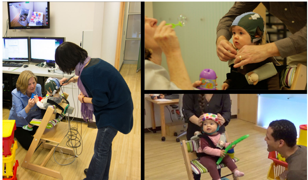
FIGURE 1 Digitization setup for use with the Polhemus device. Left panel: A toy-waver is engaging with an infant as a researcher digitizes the anatomical landmarks, head position indicator (HPI) coil locations, and additional head points. Top right panel: An infant wears a soft cap equipped with the HPI coils. Bottom right panel: A researcher places the foam halo on the infant's head before the infant is positioned under the MEG helmet
