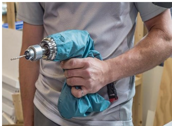
Fig. 3.7 Low-cost sterile orthopedic drill cover. (Drilling to the Problem: Low-Cost Sterile Drill Covers for Surgery 2014)
