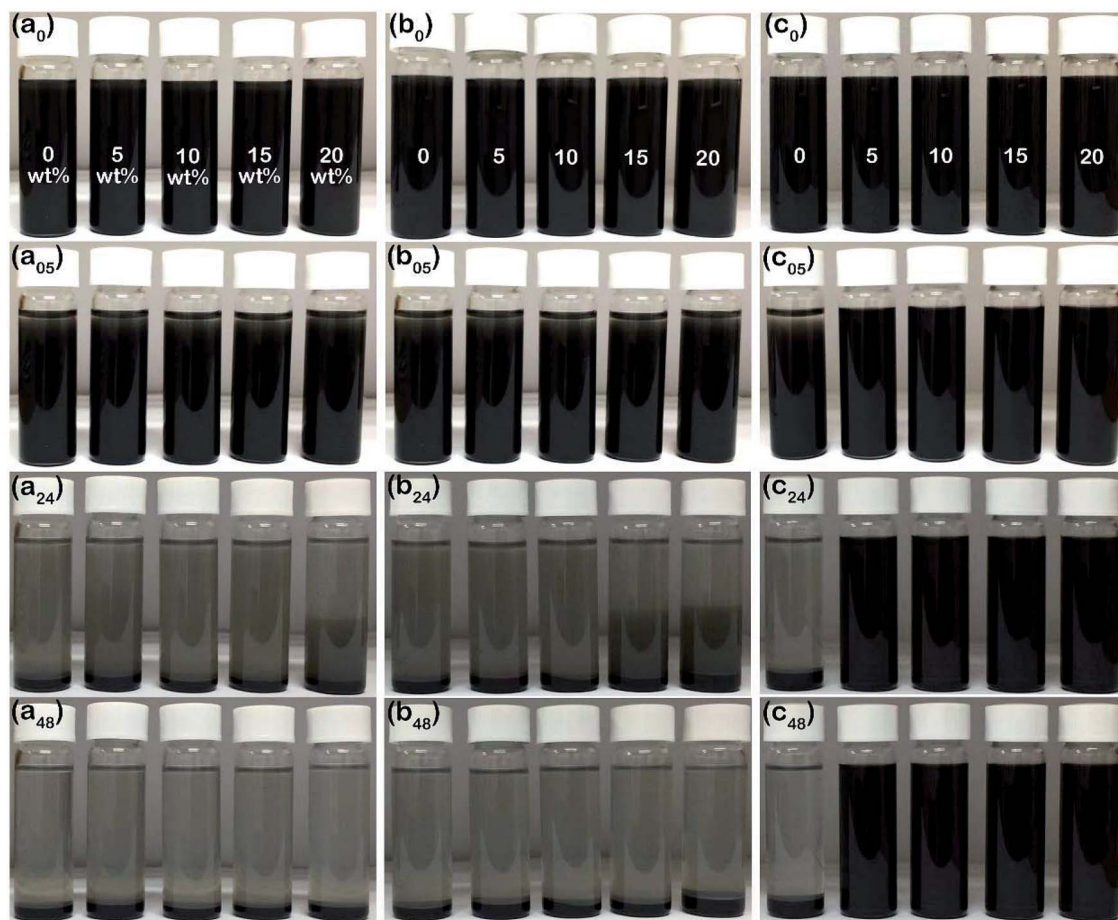
Fig. 3 Sedimentation of toluene suspensions containing 35 wt% microcapsules with the addition of (a 0 –a 48 ) OA, (b 0 –b 48 ) OP 3 , and (c 0 –c 48 ) OP for 0 min, 30 min, 24 h, and 48 h; the samples from left to right in each photo represent increasing concentration of dispersants of 0, 5, 10, 15, and 20 wt%.
