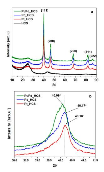
**Figure 3.** X-ray diffraction (XRD) patterns of HCS, Pd\_HCS, Pt\_HCS and Pt/Pd\_HCS. (**a**) The diffraction peaks of (111) plane in the Pt–Pd\_HCS in comparison with XRD reference data of Pt (red) and Pd (blue) (**b**).
