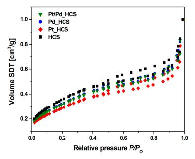
Figure 6. N<sub>2</sub> sorption isotherms of HCS, Pd\_HCS, Pt\_HCS and Pt/Pd\_HCS.
