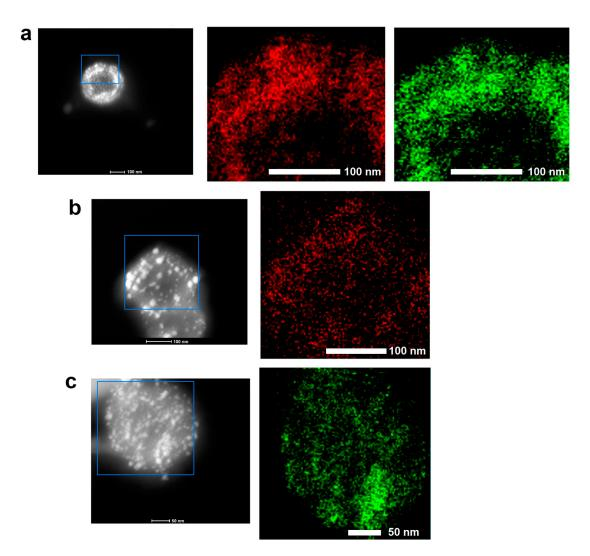
**Figure 2.** Energy-dispersive X-ray spectroscopy (EDS) elemental mapping of Pt/Pd\_HCS (**a**); Pd\_HCS (**b**) and Pt\_HCS (**c**) with the palladium (marked red) and platinum(marked green) signal. Scanning transmission electron microscopy (STEM) images with the blue square shows the scanned area.
