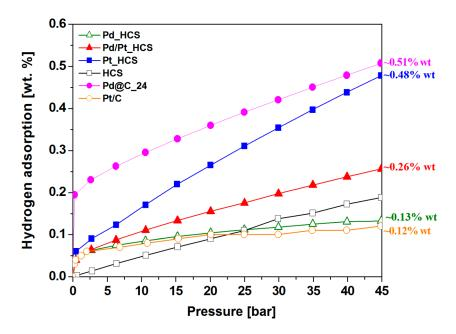
**Figure 7.** Hydrogen adsorption isotherms at 40 °C for HCS, Pd\_HCS, Pt\_HCS, Pt/Pd\_HCS, Pd@C\_24 and Pt/C.
