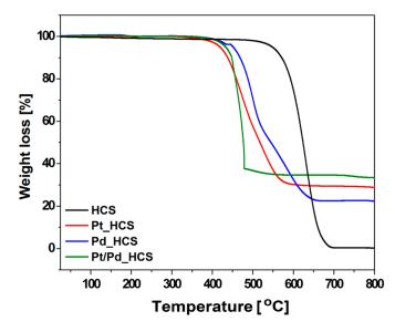
Figure 4. Thermogravimetric analysis (TGA) curves of HCS, Pd\_HCS, Pt\_HCS and Pt/Pd\_HCS.
