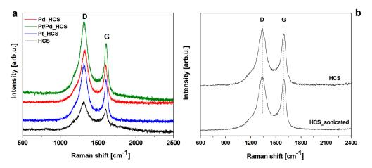
**Figure 5.** Raman spectra of HCS, Pd\_HCS, Pt\_HCS and Pt/Pd\_HCS (**a**) and comparison of the HCS and HCS after sonication (**b**).
