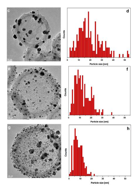
**Figure 1.** Transmission electron microscopy (TEM) images of hollow carbon spheres (HCS) (**a**); sonicated HCS (**b**) and TEM images with corresponding nanoparticles size distribution of the Pd\_HCS (**c**,**d**); Pt HCS (**e**,**f**) and Pt/Pd HCS (**g**,**h**).
