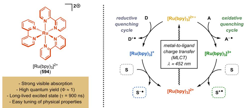
**Figure 33.** Properties of the  $[\text{Ru}(\text{bpy})_3]^{2+}$  photocatalyst (594) (bpy = 2,2'-bipyridine, MLCT = metal-to-ligand charge transfer, A = sacrificial electron acceptor, D = sacrificial electron donor, S = substrate).
