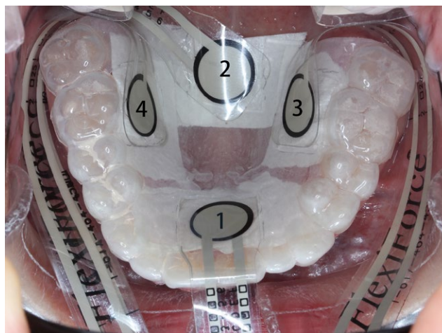
FIGURE 2 Tongue pressure measurement channel on soft occlusal pad [Colour figure can be viewed at wileyonlinelibrary.com ]
