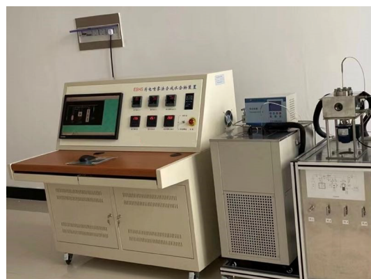
Figure 2. Physical picture of the experimental apparatus for gas hydrate formation.
