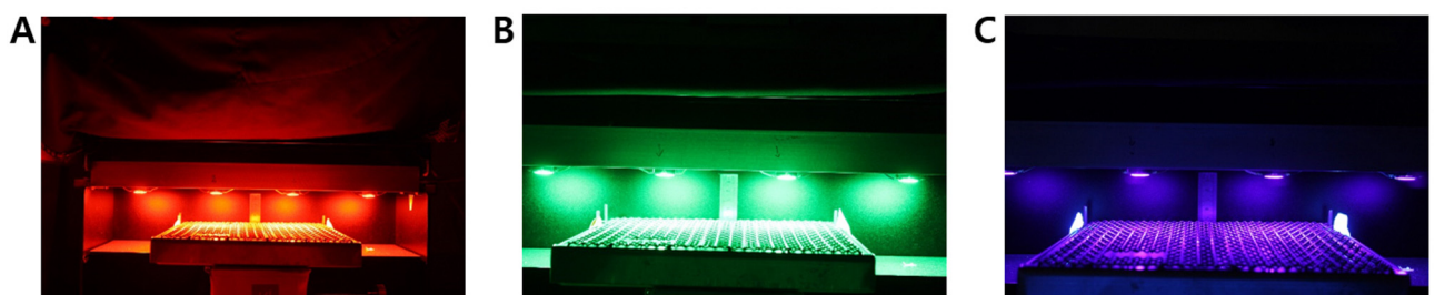
Fig 1. Light emitting diode devices and retaining cages of red light (630 nm) (A), green light (525 nm) (B) and blue light (410 nm) (C).
