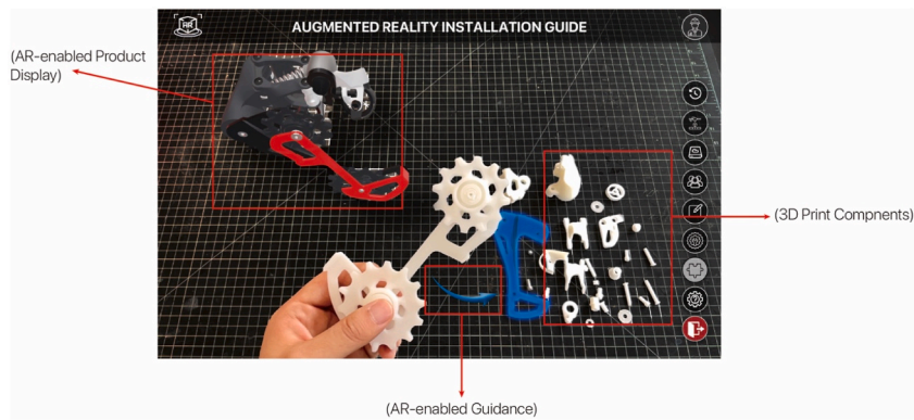
Fig. 12. AR-enabled component installation guide.
