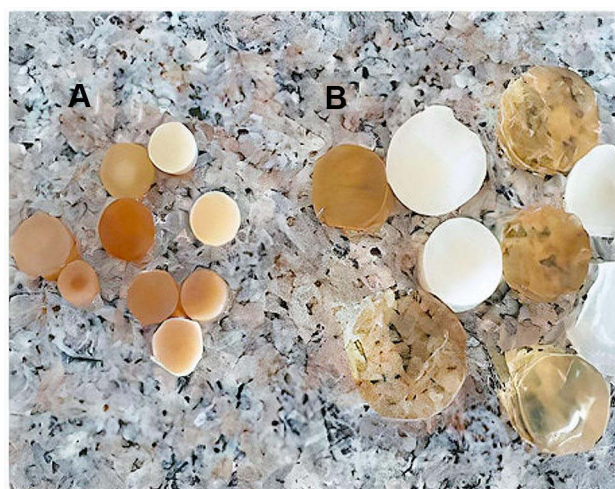
Figure 8 Swelling behavior of chitosan-co-acrylic acid hydrogels. (A) pH 1.2 and (B) At pH 7.4 Abbreviation: CH-co-AA, chitosan-co-acrylic acid.
