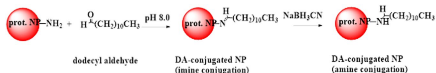
Figure 2. Conjugation of DA to proteinoid NPs showing intermediate imine conjugation.
