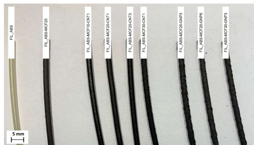
Figure 1. Extruded filaments of neat ABS, ABS/MCF, ABS/MCF/CNT, and ABS/MCF/GNP composites. Each composition is detailed in the inset.
