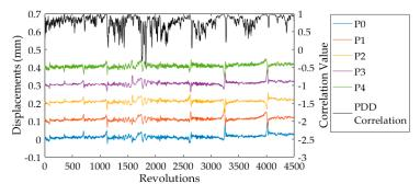
**Figure 12.** Identification results of blade 6# using the probe displacement distribution (PDD) correlation method.
