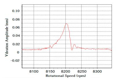
Figure 10. Model fitting result of blade 6# at 8200 rpm, engine order (EO) = 13.
