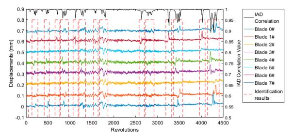
Figure 6. Identification results of blades' overall vibration events using Equation (3).
