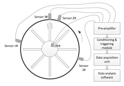
Figure 1. The block diagram of a blade tip timing (BTT) system.
