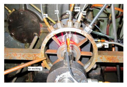
Figure 4. Test rig and installation of fiber optical tip timing sensors.
