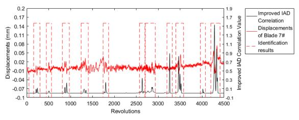
Figure 9. Identification results of blade 7# using Equation (5).
