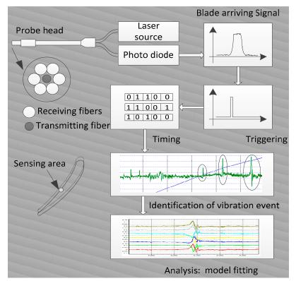
Figure 2. Signal processing of a BTT system.
