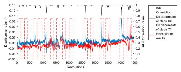
Figure 7. Identification results of blade 6# and 7# using Equation (4).
