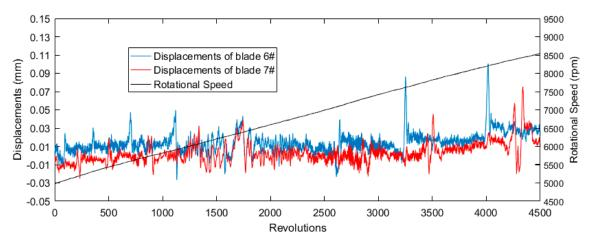
Figure 5. Blade vibration deflection and rotation speed waveforms.
