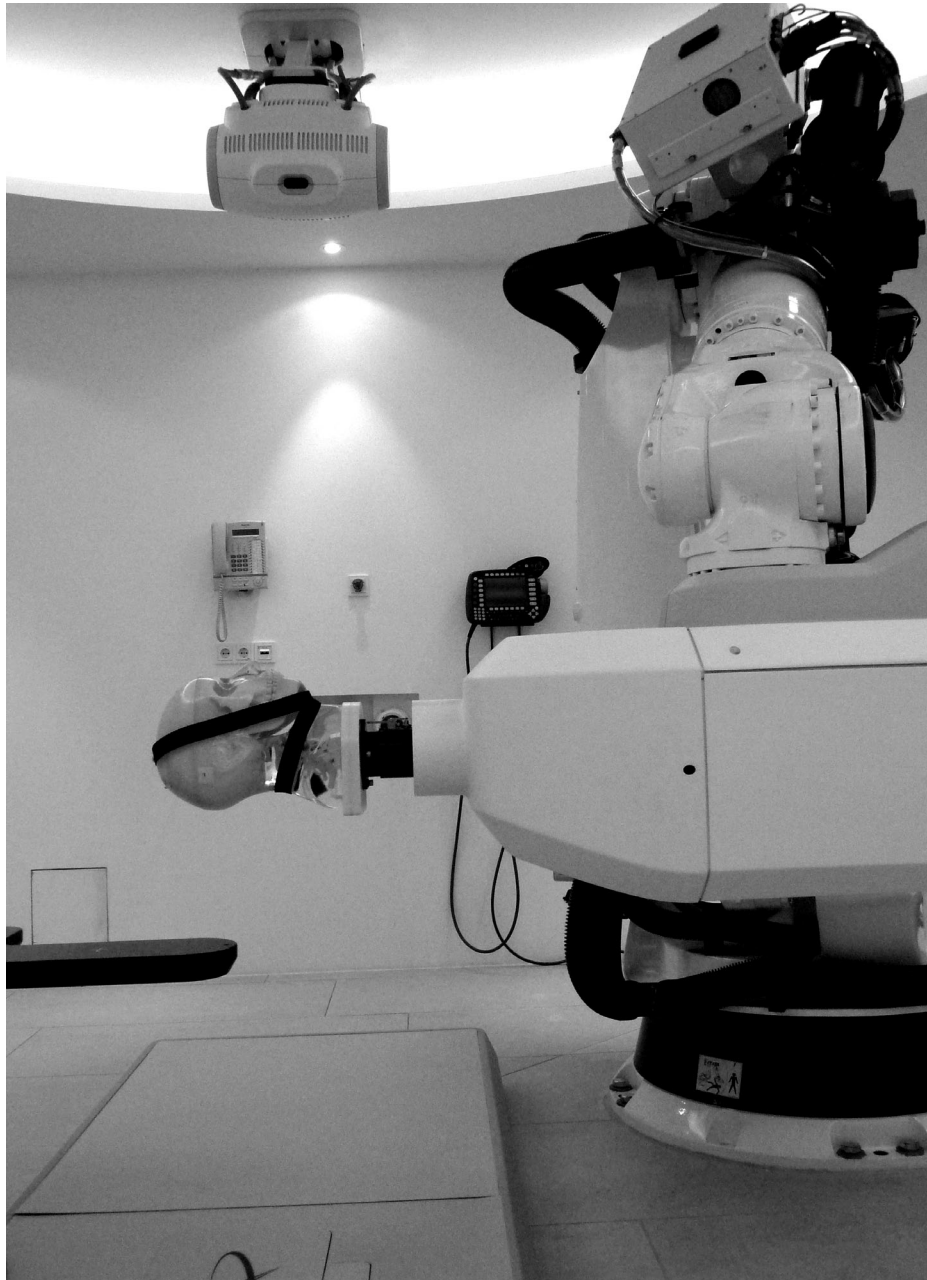
FIG. 2. Phantom tracking test setup. The socket of the anthropomorphic head-and-neck phantom is rigidly attached to the linac nozzle. Position and orientation presets of the phantom spine are reached by moving the robotic manipulator.
