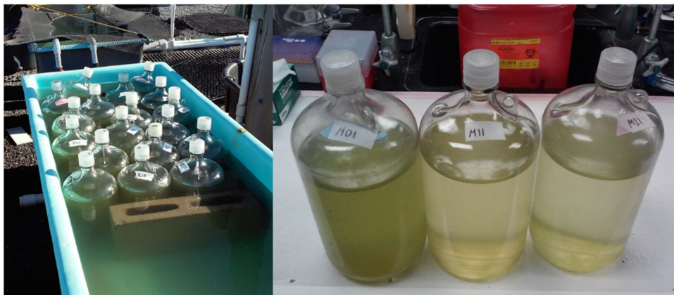
Figure 9. Outdoor flow-through table, and 4 L bottles used for incubation experiments. Example of pigment change between control and \text{H}_2\text{O}_2 treatments.
