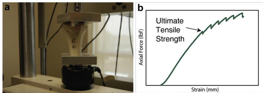
**Figure 2.** (a) Load-to-failure testing of a composite femur model with a 4-mm lateralized box and 12-mm distal resection in a universal testing machine. (b) Failure was defined as a decrease in integrity after reaching ultimate tensile strength.
