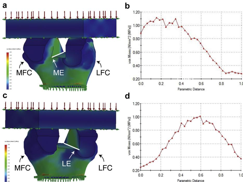
**Figure 1.** Finite element analysis of a left, size 4 femur with a neutral box cut and 8-mm distal resection under a 600-N load. von Mises stresses were measured on the (a) and (b) medial edge of the box cut and (c) and (d) lateral edge of the box cut. Maximal stresses and the corresponding parametric distance from the posterior aspect of the box edge were recorded. MFC, medial femoral condyle; LFC, lateral femoral condyle; ME, medial edge; LE, lateral edge.
