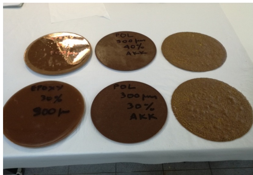
Figure 3. Composite specimens for thermal insulation efficiency testing [From left to right Epoxy Resin Composites (ERC), Unsaturated Polyester Composites (UPC), and Novolac Composites (NC) specimens].
