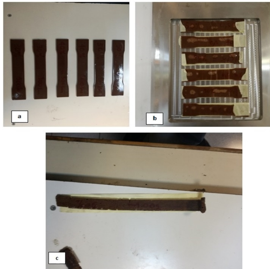
Figure 2. Specimens made for bending and shear strength tests (a) unsaturated polyester composites, (b) epoxy composites, and (c) novolac composites.
